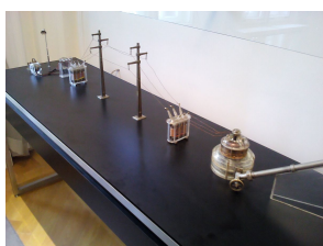
Polyphase system. Model shows example of generation, transmission and utilization of electrical energy.
