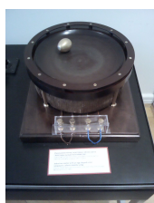
Induction motor with an egg shaped rotor, popularly called Colombo's eggs. Shown at the Exhibition on 1893 (the rotating magnetic field)
