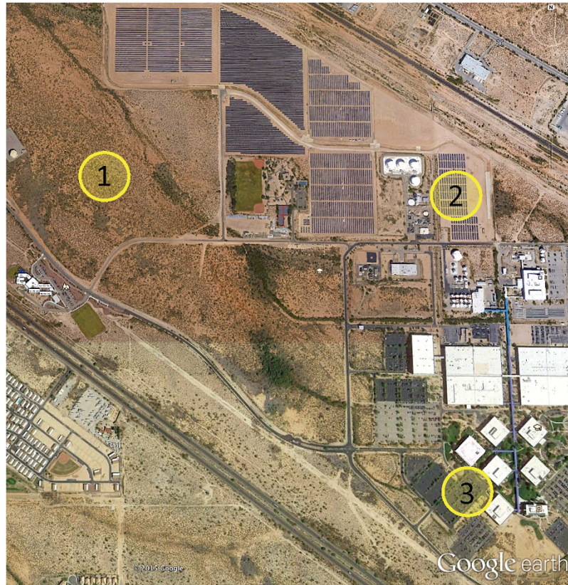
Figure 4. Experimental sites. Monitoring a (1) natural semiarid desert ecosystem, (2) solar (PV) photovoltaic installation, and (3) an “urban” parking lot – the typical source of urban heat islanding – within a 1 km 2 area enabled relative control for the incoming solar energy, allowing us to quantify variation in the localized temperature of these three environments over a year-long time period. The Google Earth image shows the University of Arizona’s Science and Technology Park’s Solar Zone.
