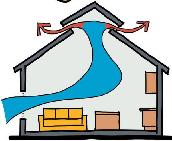
B HOT AIR ESCAPES THROUGH - CEILING
